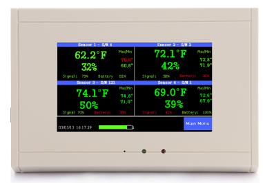
It is accurate and automatic, providing continuous monitoring and indicating trends so that corrective action can be taken. In addition to the display showing the current temperatures, it can also show a chart on the large LCD display.
