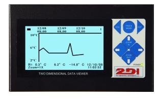
A quick look at the large display is all that is needed to insure that the proper temperature has been maintained over the last day, week, month or year. It shows the current temperature and over a year of temperature history for two different freezers. Its relay will trigger the audio/visual alarm and the optional auto dialer if the temperature gets too warm or cold.
